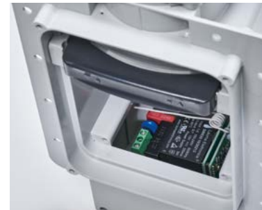
Receiver installed in the backplate of the Sense system
